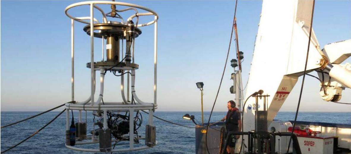
**Carousel Water Sampler being lowered into the water column structure across the Project area**
