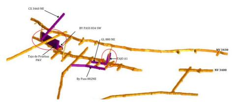
The following diagram further shows all the stopes that these two existing sub-levels would have allowed to extract in Year 1 of production:<sup>117</sup>
